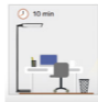
After another 10min, the lamp switches off when motion is not detected
